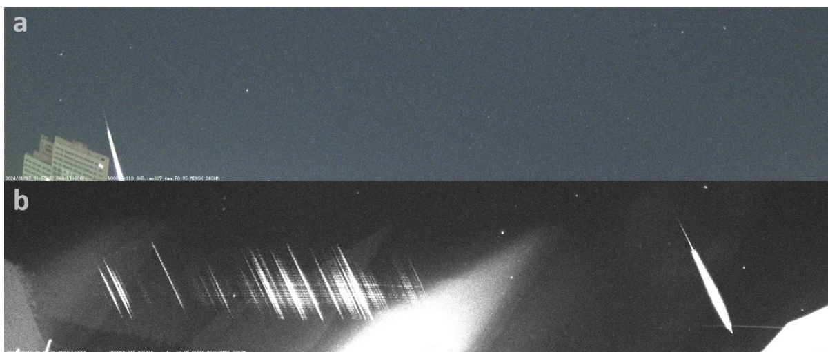
Figure 1 – Images of the meteor captured by the Minsk_24 camera (a) and the Derazhnoye_30 spectral camera (b), which shows the original image with a first-order diffraction spectrum. The spectral image also shows diffraction grating-induced stray light from a bright terrestrial object (illuminated rooftop).
